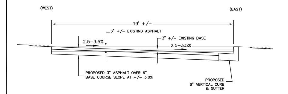
CONSTRUCTION NOTES: REMOVE EXISTING ASPHALT
