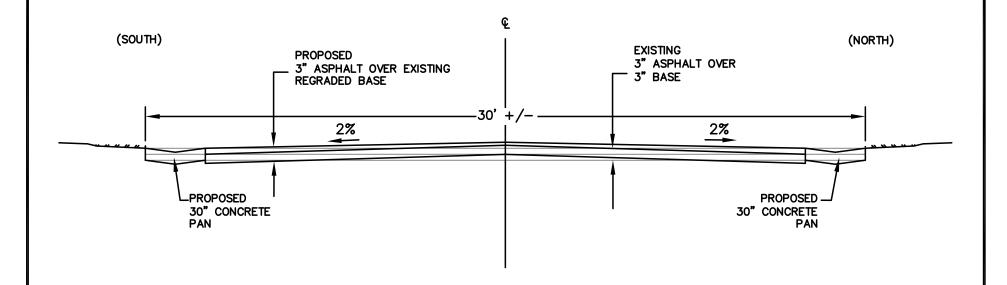
CONSTRUCTION NOTES: REMOVE EXISTING ASPHALT
