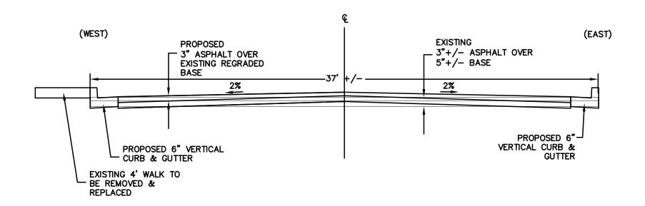
CONSTRUCTION NOTES: REMOVE EXISTING ASPHALT
